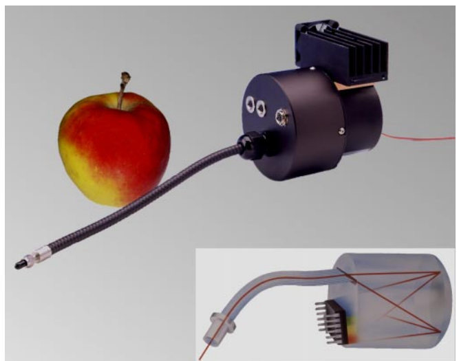
Fig. 1: MMS-NIR 1.7 (Carl Zeiss Jena GmbH) dismounted (top) and in schematic view (bottom)
